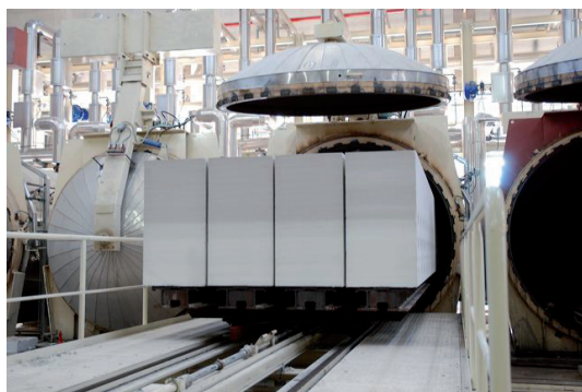
Optimised autoclave loading in Wehrhahn PLUS plant
