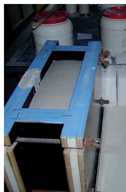
Fig. 2. The moulds used for green cake expansion (left) and the set-up used for monitoring (right).
