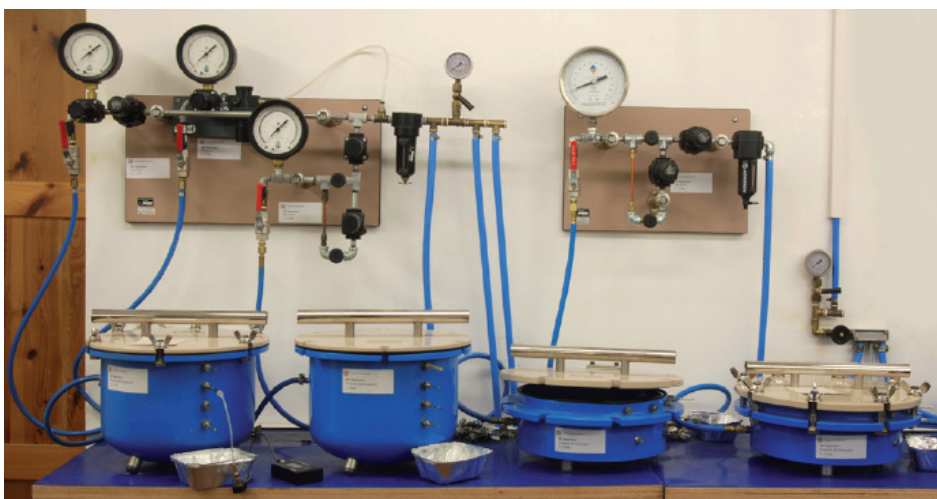
Fig. 2. Pressure plate apparatus consisting of two 5 bar and two 15 bar pressure chambers.
