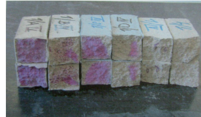
Fig. 8. Concrete specimens after half year acting of CO 2
