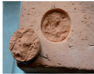
Fig. 13. Cohesive failure of silicate adherend
