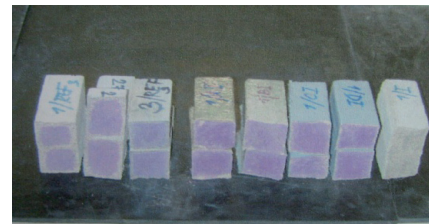
Fig. 7. Concrete specimens after starting assessment on CO 2 penetration
