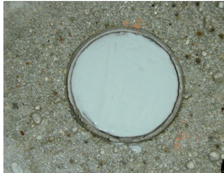
Fig. 1. Application of adhesive L1 on ground concrete substrate
