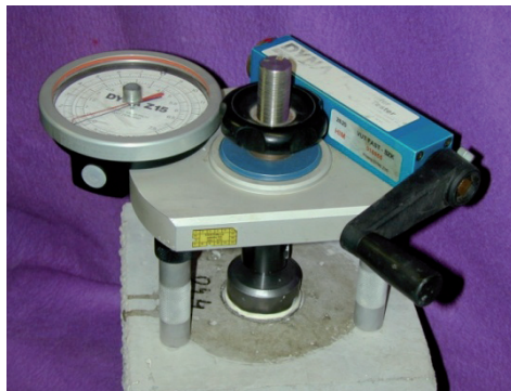
Fig. 2. Testing apparatus Dyna Z 15 made by PROCEQ Company
