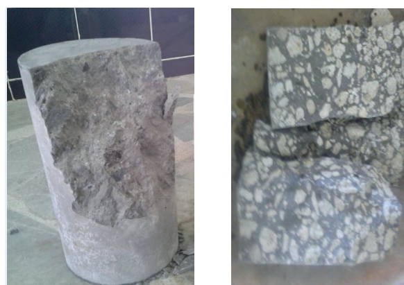
Fig. 4. Test cylinders of conventional (left) and pumice lightweight concrete (right) after compressive strength measurements
