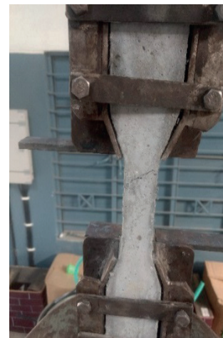
Fig. 3. Failure pattern of ECC after tensile strength measurement
