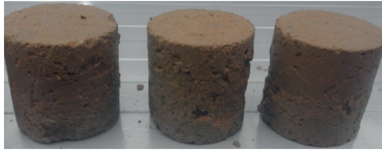
a) Pg stabilizowany cementem z dodatkiem 7% mleczanu diamidoaminy / Pg stabilised with cement with a 7% addition of diamidamine lactate
