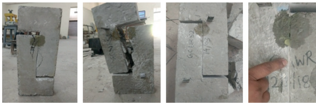
Fig. 4. Failure pattern for unreinforced and reinforced across shear plane
