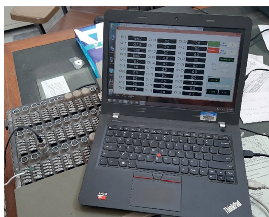
(b) Data logger setup for data acquiring from the UTM and digital dial gauge for lateral deformation measurement
