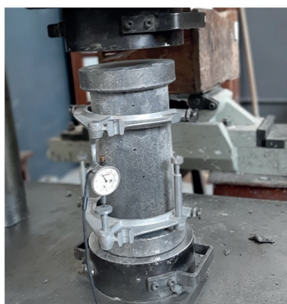
(a) Digital dial gauge for lateral deformation measurement installed on standard Cylinder specimen.
