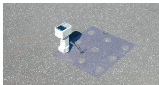
Fig. 5. Measuring arrangement to determine the level of reflectance [Picture: SMG – Smart Minerals GmbH]
